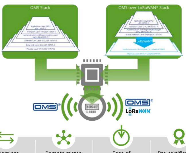
Seamless switching between stacks ensures maximum flexibility Remote meter reading enabling fixed networks and walk-by/drive-by
