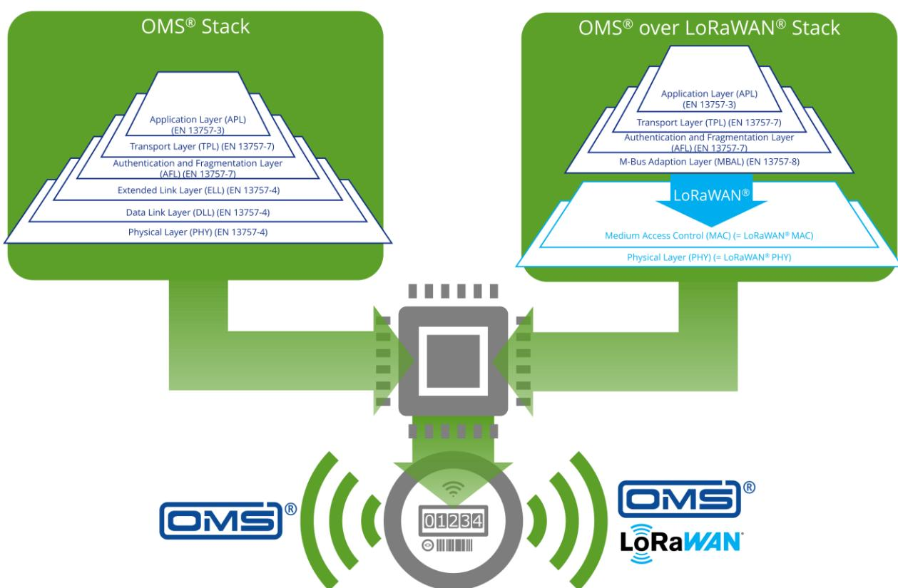
Seamless switching between stacks ensures maximum flexibility
