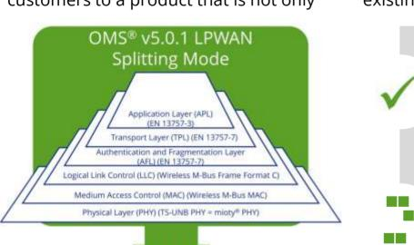
characterized by excellent robustness thanks to the integration of telegram splitting technology, but also has a significantly greater range than previous OMS<sup>®</sup> versions.
